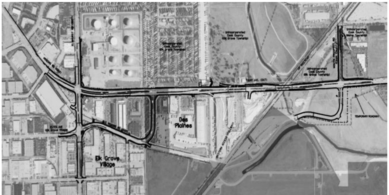
Figure 18: Map of Touhy Avenue improvements. This project reduces congestion and improves reliability through a new grade separation at the Union Pacific Railroad and intersection improvements at Elmhurst Road.
