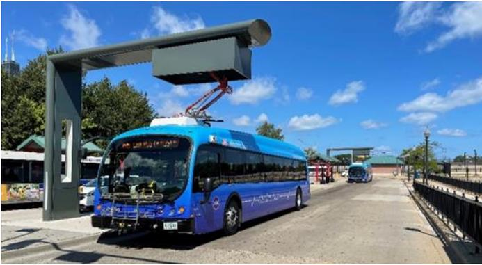
A CTA electric bus charges using the high-powered, overhead charger at the Navy Pier bus-turnaround.
